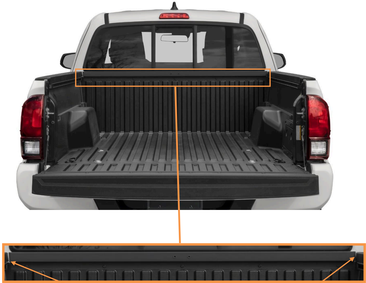
Fig 12: Gaps in Factory Bulkhead Spacer
