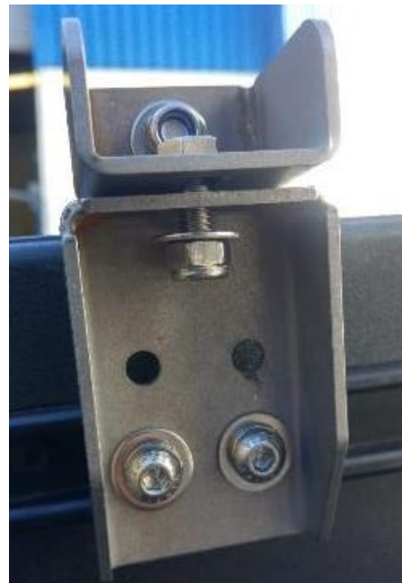
Fig 11: Photos of Bracket kit assembled in Tacoma Load Bin
