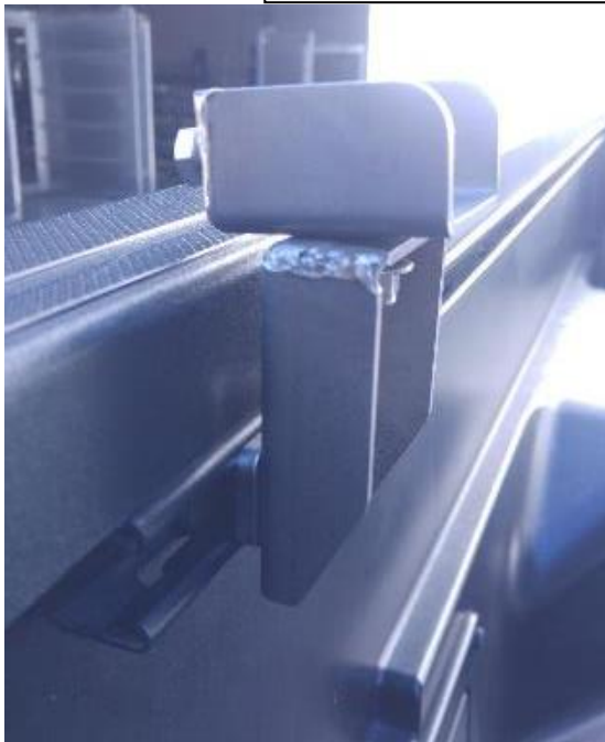
Fig 11: Photos of Bracket kit assembled in Tacoma Load Bin
