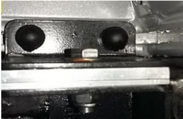
Figure 19: Front Support Bracket Installed
