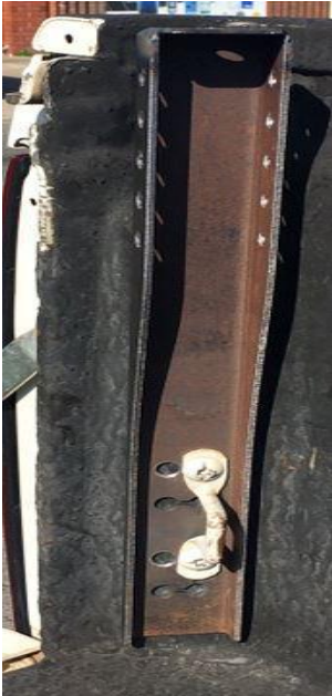
Figure 13: Rear Bracket installed
