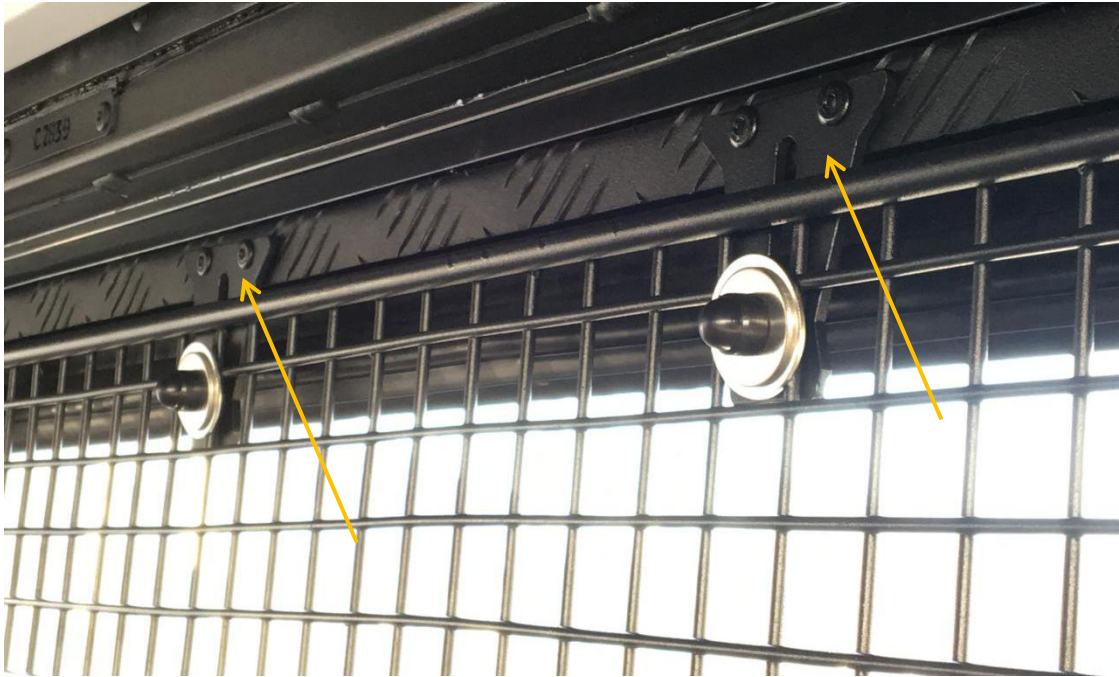
Figure 8: Top Vertical Mounts drilled and riveted to the Top Aluminium lip on the Canopy Rear Door.
