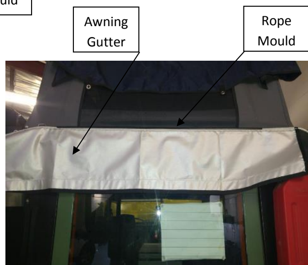
Figure 12: Gutter Installed into Rope Mould
