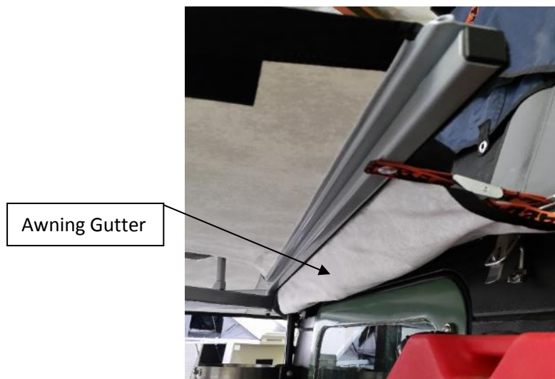
Figure 14: Awning Gutter Fully Installed
